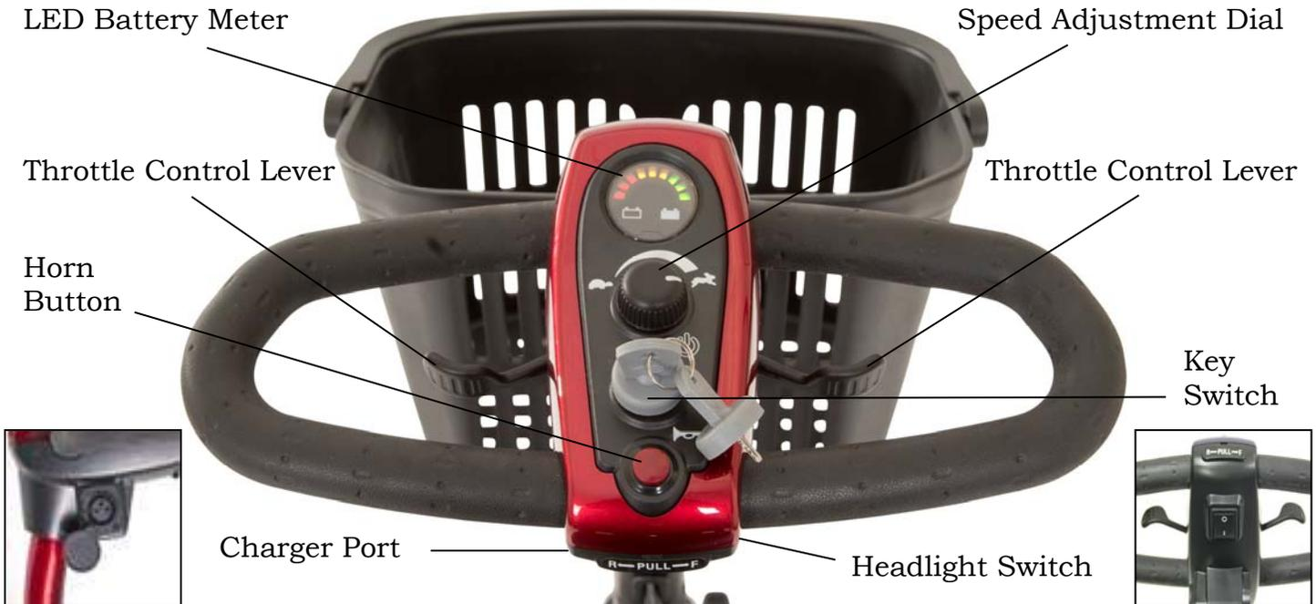
**Figure 5. LiteRider™ Delta Tiller Control Panel**
