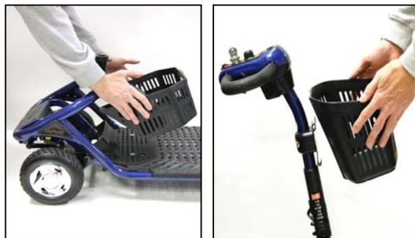
**Figure 15. Removing the Baskets**
