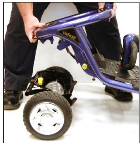
**Figure 18. Lifting the Frame**
