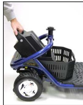
**Figure 14. Removing the Battery Pack**
