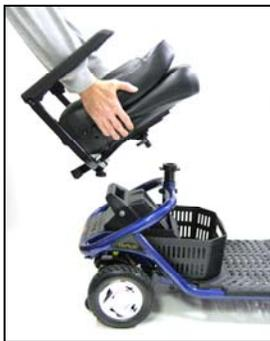
**Figure 13. Removing the Seat**
