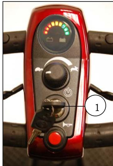
**Figure 12. Key Switch (On)**
