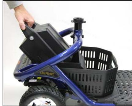
**Figure 21. Battery Pack Installation**
