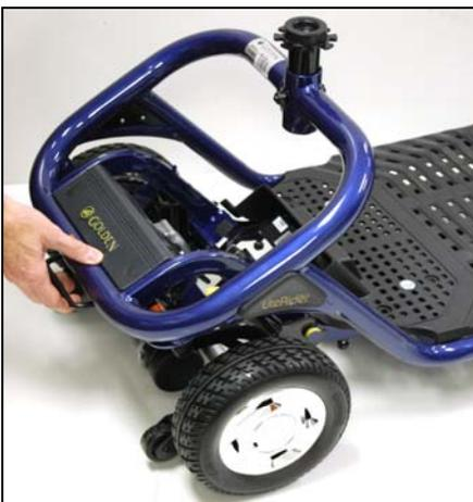
**Figure 17. Releasing the Drivetrain**
