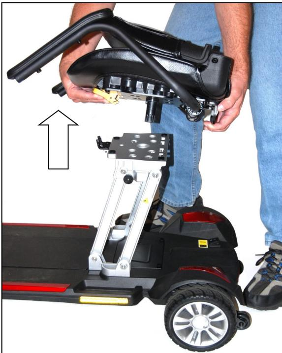
**Figure 12. Removing Seat**
