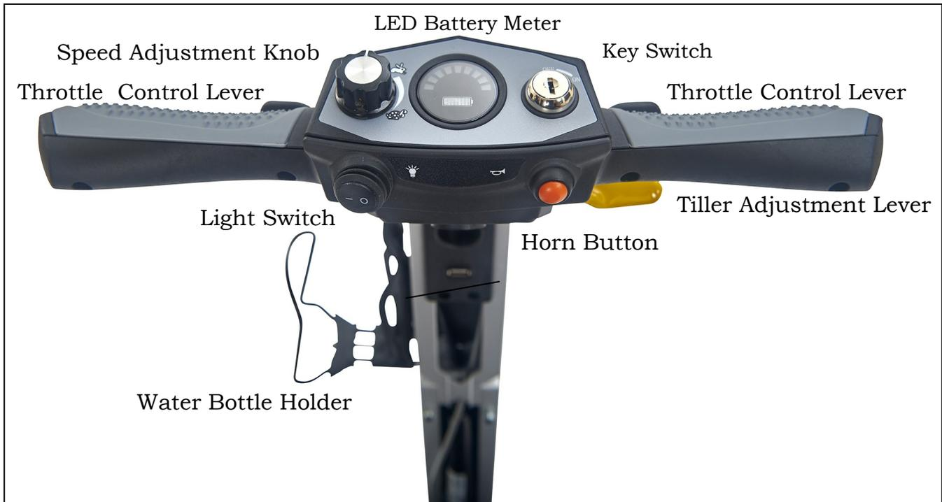
**Figure 5. Carry On Tiller Control Panel**
