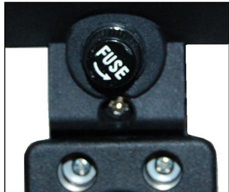
**Figure 27: 3 AMP Tiller Fuse**
