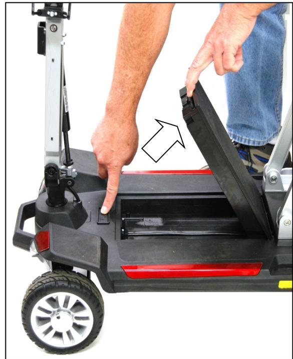
**Figure 13. Removing Battery Pack**
