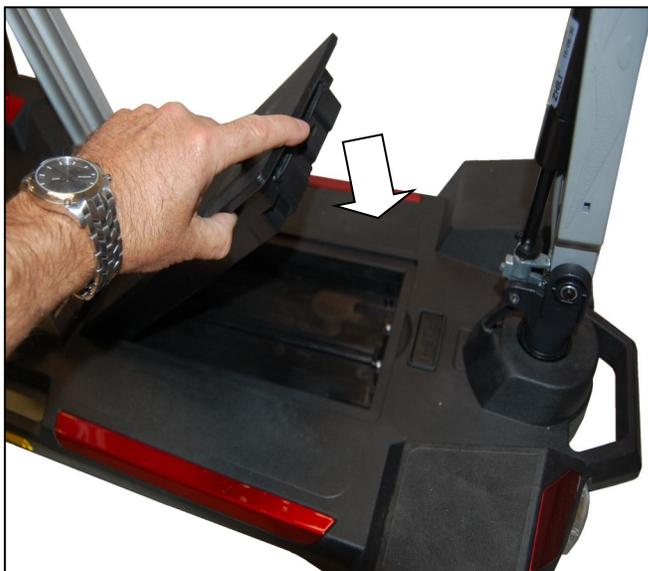
**Figure 20. Installing Battery Pack**
