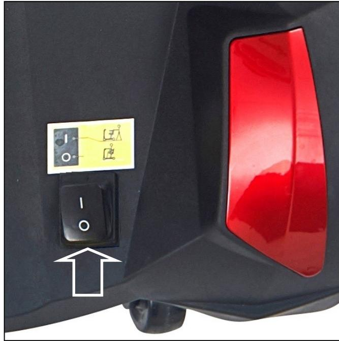
**Figure 9: Freewheel Switch (Drive Position)**
