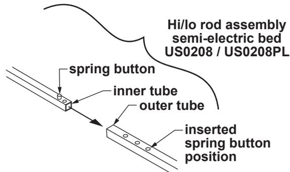
Depress spring button and insert inner tube into outer tube until third hole is reached as shown above. Release spring button to lock it into hole.
