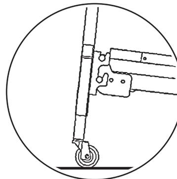
5. Engage lower rivet slightly with corner lock and tilt end toward bed as shown at above left.
