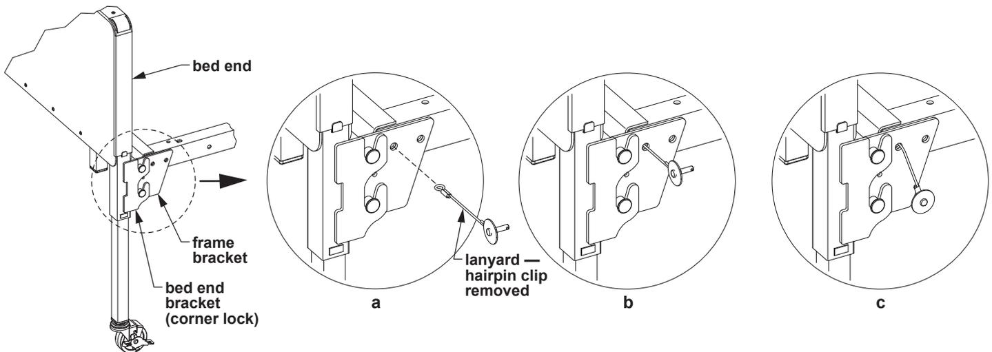
2. Refer to accompanying illustrations while installing Bed End Locking Hardware. Remove the hairpin clip from the end of the lanyard assembly, as shown in **a**, and set it aside.
