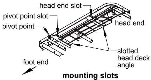
The Half No-Gap Head Rail, shown above, provides full head coverage of 31.5 inches and extends to eliminate the gap between the head board and the end of the rail. The GF6590BH-1 mounted on the bed's head and the GF6580BH-1 mounted on the bed's foot combine to create the Patriot split rail system.
