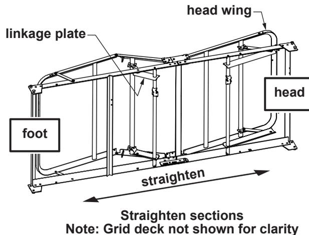
3. With the rivets fully seated in the hooks as described in step 2, rotate and straighten the bed as shown above. Position head wing as shown above.
