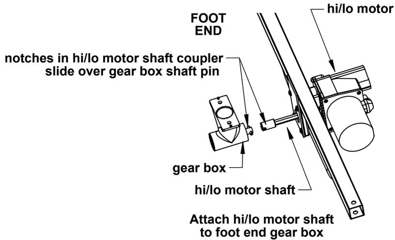
You must first attach the coupler end of the motor shaft to the foot-end gear box (see above).
