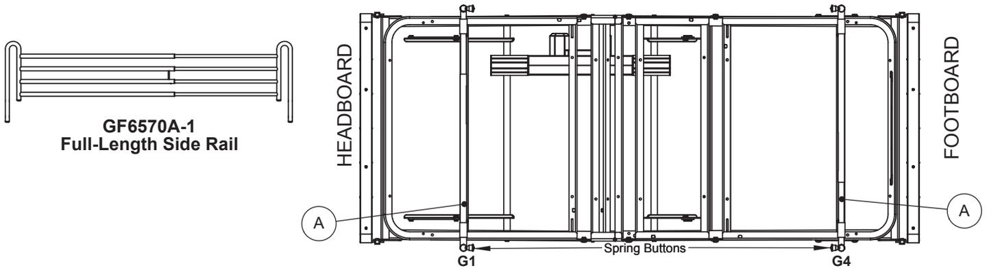
Position spring-loaded crossbraces #A into slots G1 and G4 on both sides of bed with spring buttons facing inward as shown above.
