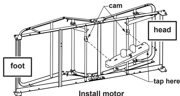
3. Hold the bed securely, positioned with motor cams up, as shown above.
