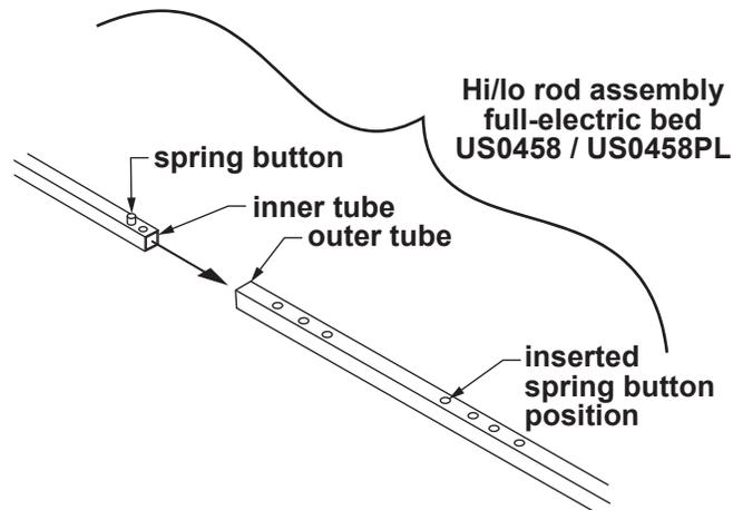
Depress spring button and insert inner tube into outer tube until first hole of second hole set is reached as shown above. Release spring button to lock it into hole.
