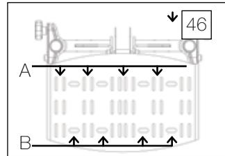
46B. **Foot Holders**-Position foot holders into desired position. Insert bolt and tighten knob securely.
