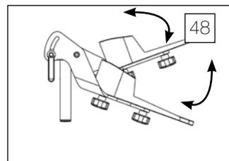
49. **Abduction**-Loosen knobs to slide foot plates together. Tighten knobs securely
