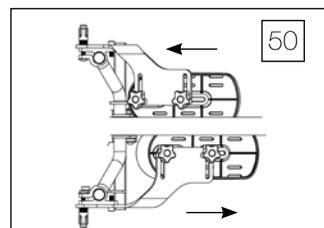
51. **Toe-in/Toe-out**-Loosen knobs underneath foot plates, slide foot plates into position. Tighten knobs securely
