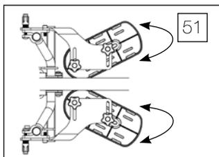
52. **Abduction**-Loosen ratchet handles to spread apart foot plates, tighten securely. Loosen knobs under foot plates and slide foot plates apart. Tighten knobs securely
