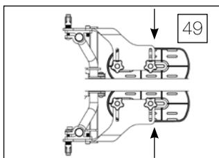
50. **Forward/Aft**-Loosen knobs underneath foot plates, slide foot plates into position. Tighten knobs securely
