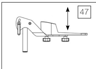
48. **Plantar/Dorsi**-Loosen ratchet handles to tilt foot plates. Tighten securely.
