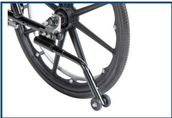
2. To use optional 12" rear wheels remove axle plate bolts, move axle plate to forward position, below the frame rail. Re-install bolts and tighten to secure. Depress quick release axle button and slide axle into axle sleeve.
