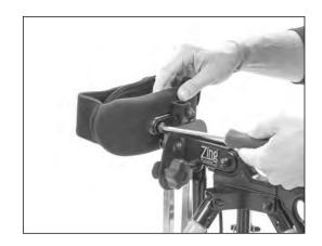
8. Place upper body support bracket into tube as shown. Depress the spring button.
