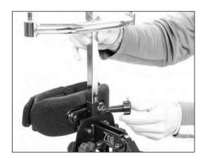
10. Remove 2 small knobs and washers from the parts bag. Place washer onto the tray bracket as shown.
