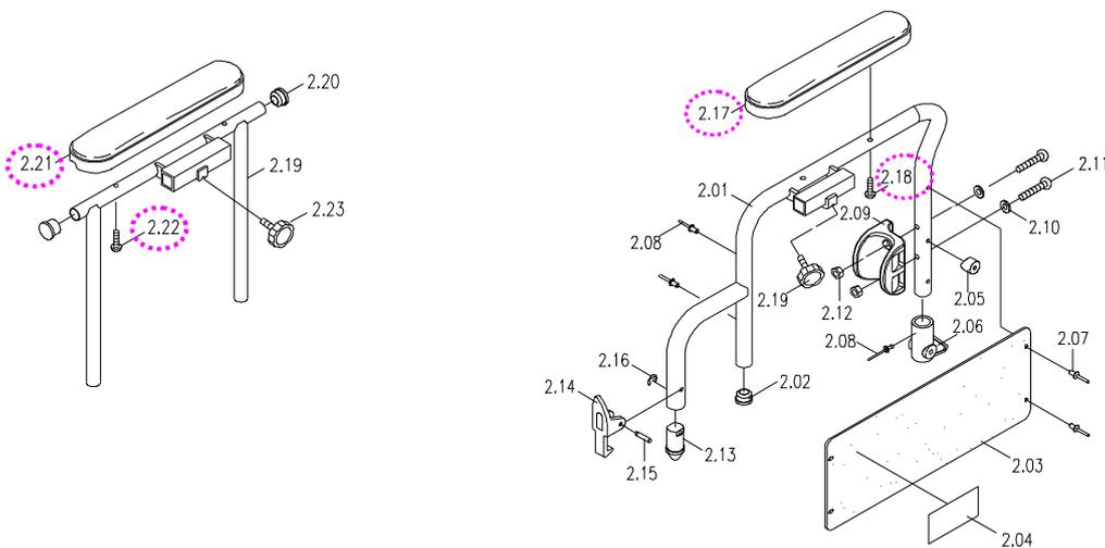
2. Use hex. tools and wrench to loosen the screw (1.08) and nut (1.05) from bracket (1.07) on the side frame (see page 14). If the armrest assembly (2.1) is worn out or deformed, then replace it.
