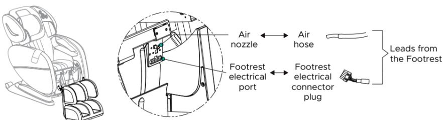
**17 Step 17:** Lift up and pull back flap on the footrest. Slide the footrest in and shift it until the mounting bracket is properly aligned with the screw holes located on the chair body. Insert the hex screws through the screw holes to fasten the footrest to the body of the chair. Repeat on other side. Tighten with Hex Key.
