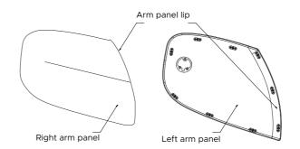
To attach the arm panels, align the connectors on the arm panels with the sockets on the chair body. Push firmly to connect into place.
