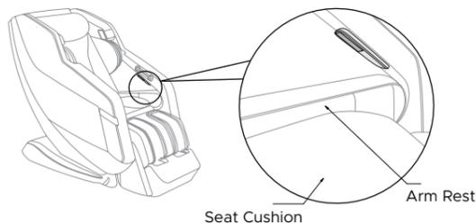
**8 STEP 8:** The arm rest of your chair comes with a unique feature: swing the arm rest up to reveal an arm massage sleeve. Once you are done, swing the arm rest back down to use it again as an arm rest.
