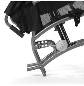
The further back the axle mounts are installed, the less likely the wheelchair is to tip over in use, i.e. in this configuration there is the least likelihood of the wheelchair tipping backwards. The further forward the axle mounts are installed, the lower the proportion of the total weight that is over the forward casters, making it easier to deliberately tip the wheelchair backwards (either by the user or the companion), which in turn makes the chair easier to maneuver.
