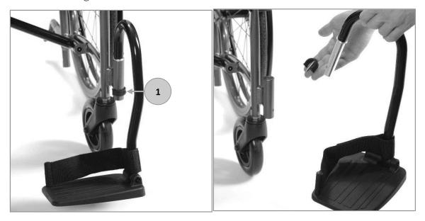
The footrests can be completely removed from the wheelchair by pulling the plastic clip with its retaining pin (1) horizontally out of the tube. The whole of the footrest can then be pulled up and out of the footrest mounting. When refitting the footrests ensure that the hole for the locking pin in the footrest is aligned with the hole in the frame.
