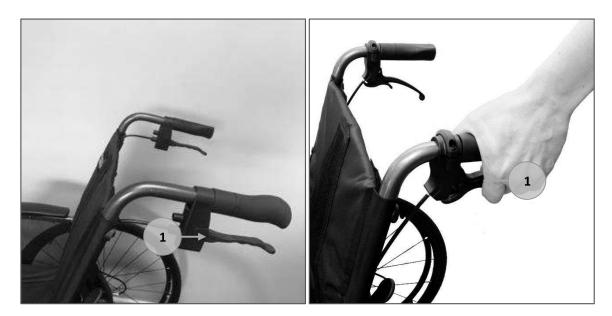
The attendant brakes can be locked in one of the following two ways (depending on the type of attendant brake installed on your wheelchair):
