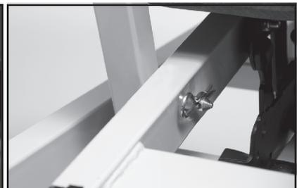
8. Raise the upholstered back to vertical position. Tuck the plastic skirt at rear of upholstered back behind cross brace of seat frame. Align the hinges at the bottom of the gas spring with the holes in the U-brackets on the seat frame cross brace. While holding the back in position with one hand, secure the gas spring hinge to the U-bracket by placing the 5/16" diameter clevis pins through the U-bracket and hinge with the other hand.
