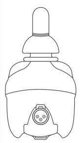
Plug the battery charger into the charging socket loocated at the front of the SHARK Control Unit.
