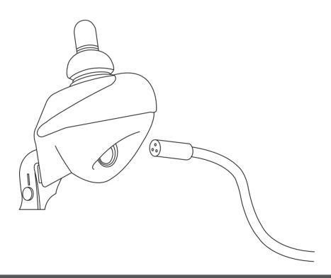
WARNING: Do not exceed the maximum charging current of 12 A rms. Always use an off-board charger fitted with a Neutrik NC3MX plug. Failure to observe these conditions could result in poor contact resistance in the charger connector resulting in overheating of the charger plugs. This presents a potential burn hazard for the user. Penny & Giles accepts no liability for losses of any kind rising from the failure to comply with this condition.
