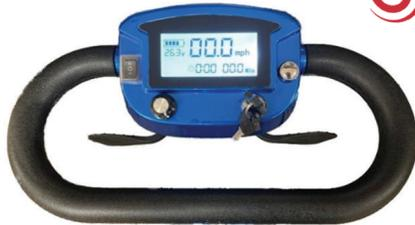
The informative LCD Display shows the battery level, battery voltage, speed you are traveling at and distance.
