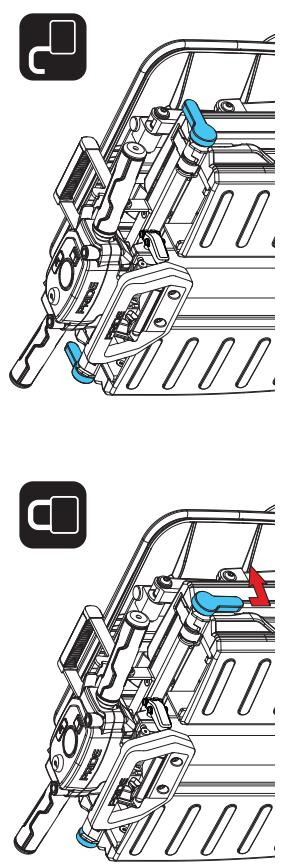
**NOTE:** To refold scooter, remove key, ensure the manual freewheel lever is in drive mode, and reverse steps 1 through 5.
