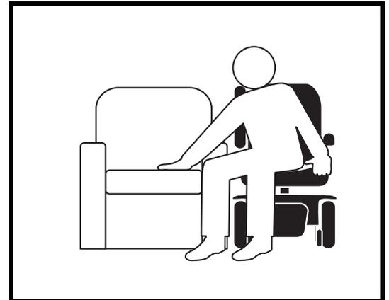
Figure 8. Recommended Transfer Position
