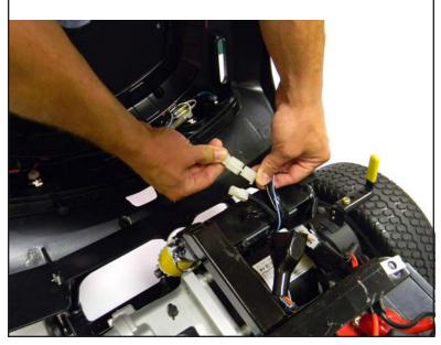
**6.** Replace the rear shroud and reinstall the two knobs removed in Step 2.
