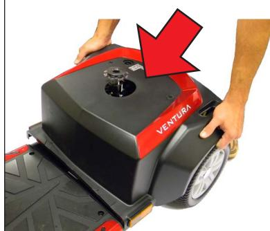
While lifting up on the seat release lever, place the seat onto the seat post. Release the lever and rotate the seat until it locks into place.
