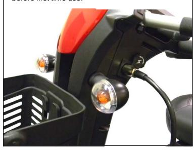
If equipped (DLX models), secure the mirrors to the tiller by inserting the mirrors into the connections points on either side of the control panel and rotate clockwise until secured into position.
