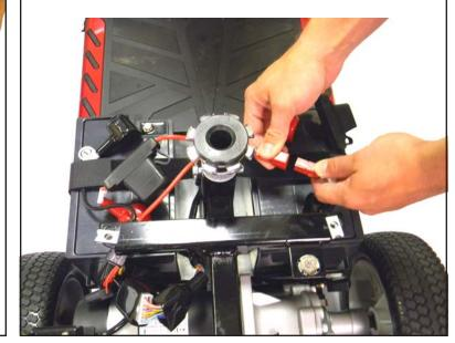
If equipped (DLX models), connect the rear light harness on the rear shroud to the main cable on the base of the scooter.
