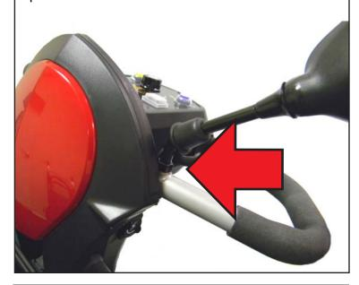
Before use, make sure that the scooter's yellow freewheel mode lever is in the "drive" position.
