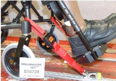
Fitting the front restraint
