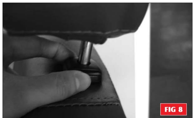
To lock the handlebar into a comfortable driving position, simply push the black lever downwards until the handlebar is locked firmly into position. With the combination of the height adjustment together with the handlebar movement, you should find a suitably comfortable driving position.
