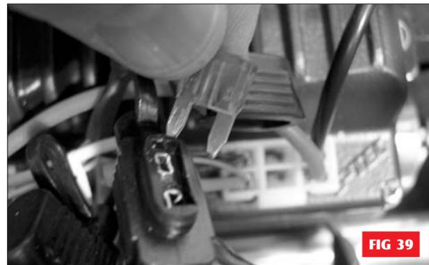
For access to a fuse remove the four screws located in the rear body cover, lift cover. Locate and lift the fuse block on it's wire, lift up the fuse lid and withdraw the 'read' fuse. Replace the blown fuse with recommended 10amp (pink) fuse, close fuse lid and replace fuse block.
