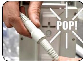
Make sure the contact point of the control box and the battery are not damaged or corroded. If there is corrosion clean with Scotch-Brite™ pad. Put some dielectric grease on the contact points before reattaching the battery.
