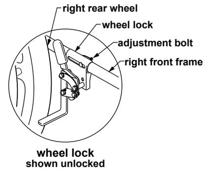
**⚠ WARNING: Ensure wheel locks are adjusted so they lock in place appropriately before occupying or operating wheelchair.**
