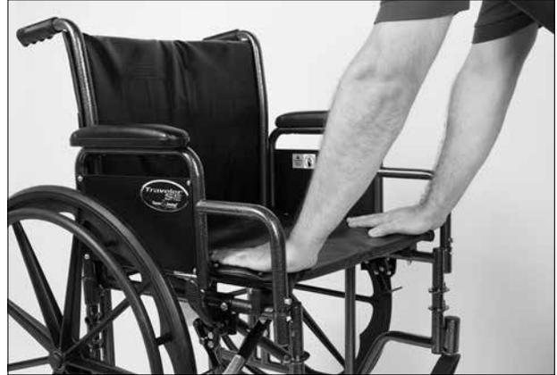
2. Use both hands to push down with even pressure on seat tubes and seat upholstery on insides of wheelchair, as shown at above left, until the seat rails are fully seated, as shown at above right. ***Do not place any fingers or parts of your hand under the seat rails.***
